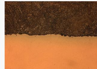
The Dycobond® technology makes it possible to produce a spatial composite of materials with different thermal expansion properties. The result is an excellent, high-strength and sealed diffusion bond.
