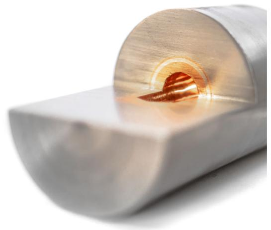
The Dycobond® process revolutionizes the internal mold cooling by inserting a thick, multilayer lining into the cooling channel made in a single working step directly during the hardening process.
